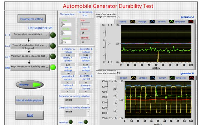
Fig. (4). Front panel of user interface.
