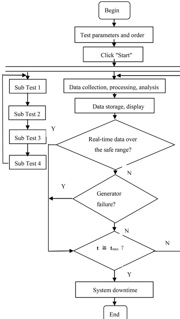
Fig. (3). Durability test work control process.
