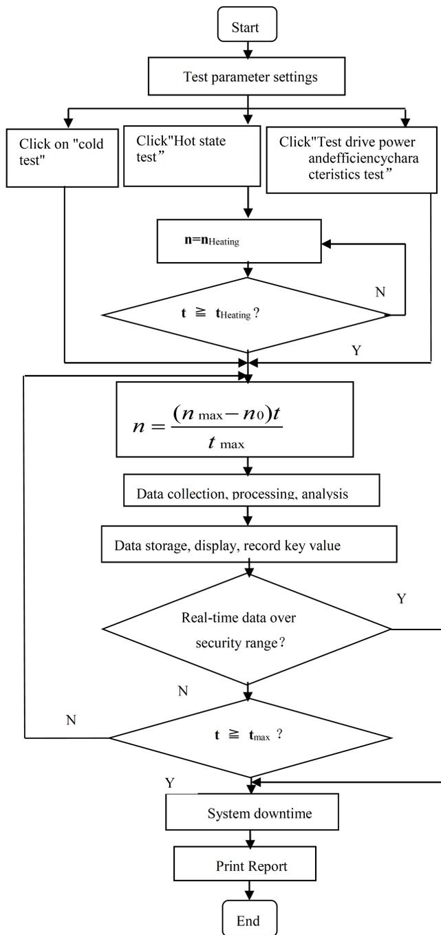
Fig. (5). The electrical characteristics of the test control flowchart.
