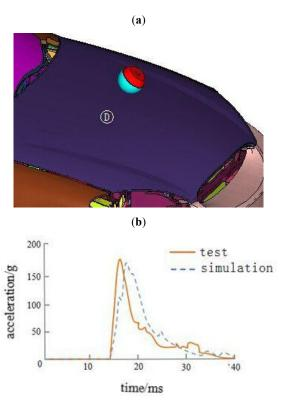
Fig. (3). Validation simulation (a) test setting (b) acceleration comparison of test and simulation.
