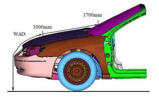
Fig. (1). Finite element model of the sedan front structure.
