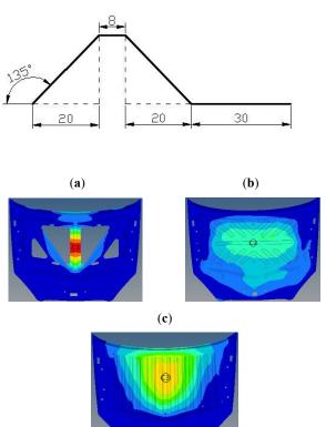
Fig. (9). The energy contours at collision point C3 (a) original structure (b) radial stiffener structure (c) trapezium sandwich.
