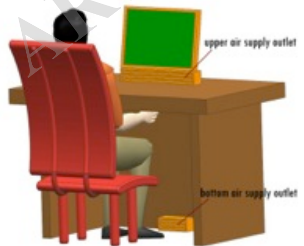
Fig. (1). Desk personalized ventilation model.
