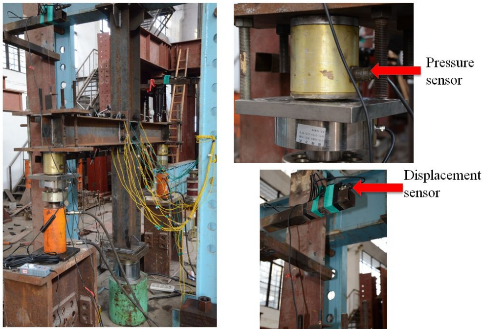
Fig. (3). Arrangement of pressure sensor and displacement sensor.
