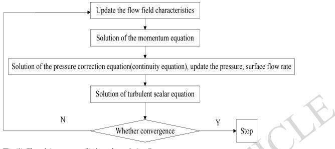
Fig. (1). The solving process of independent solution diagram.
