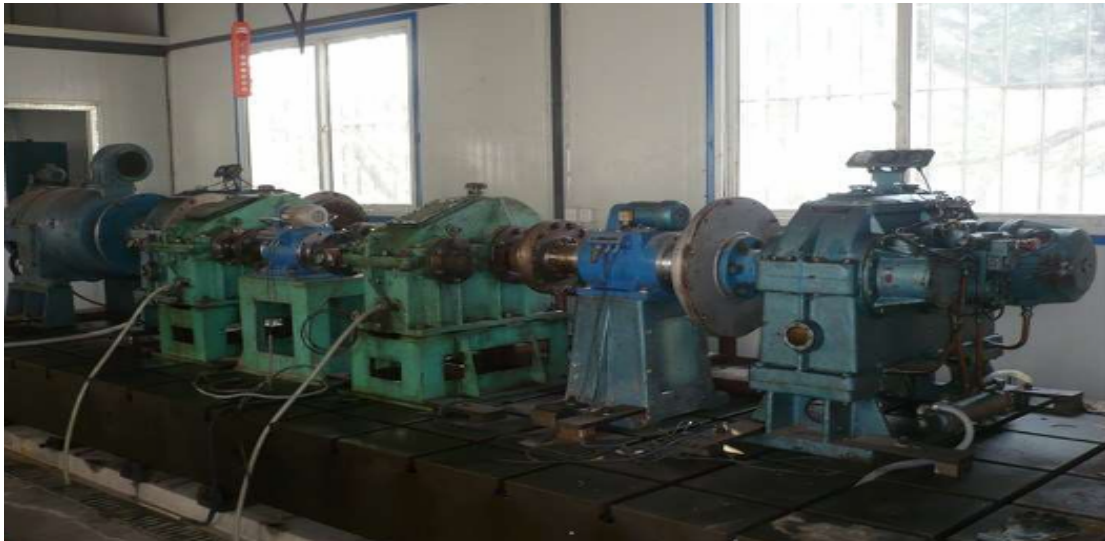
Fig. (21). Hydraulic loading test bench of helical gear.
