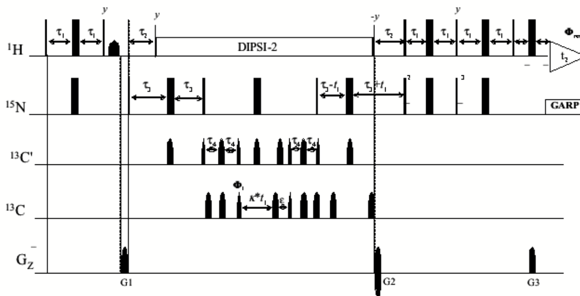
Figure S2. R.f. pulse scheme of GFT (3,2)D HNN(CO)CA. Rectangular 90^\circ and 180^\circ pulses are indicated by thin and thick vertical bars, respectively, and phases are indicated above the pulses. Where no r.f. phase is marked, the pulse is applied along x . High-power 90^\circ pulse lengths are: 10.0 \mu\text{s} for ^1\text{H} , 35 \mu\text{s} for ^{15}\text{N} and 14.8 \mu\text{s} for ^{13}\text{C} . \kappa=0.5 (see text). The ^1\text{H} r.f. carrier is placed at the position of the solvent line at 4.7 ppm. The ^{15}\text{N} carrier position is set to 121.0 ppm. The ^{13}\text{C}' carrier is placed at 176 ppm before the first pulse on ^{13}\text{C}^\alpha and shifted back to 176 ppm after the last 90^\circ r.f. pulse on ^{13}\text{C}^\alpha . A Gaussian shaped ^1\text{H} r.f. pulse [1] of length 1.0 ms is used for water flip-back prior to the first r.f. pulse on ^{15}\text{N} . DIPSII-2 [2] is used for ^1\text{H} decoupling during heteronuclear transfer periods. GARP [3] is employed to decouple ^{15}\text{N} (r.f.=1.50 kHz) during acquisition. All pulsed z-field gradients (PFGs) are sine-bell shaped with gradient recovery delay of 200 \mu\text{s} . The duration and strengths of the PFGs are: G1 (0.5 ms, 30 G/cm); G2 (2.0 ms, 40 G/cm); G3 (2.0 ms, 4 G/cm). The delays are: \tau_1 = 2.3 \text{ ms} , \tau_2 = 5.5 \text{ ms} , \tau_3 = 12.5 \text{ ms} , \tau_4 = 4.0 \text{ ms} . Phase cycling: \phi_1 = x ; \phi_2 = 2(x), 2(-x) ; \phi_3 = 2(y), 2(-y) ; \phi(\text{receiver}) = x, -x, -x, x . A sensitivity enhancement scheme [4] is employed, i.e. , the sign of G2 is inverted in concert with a 180^\circ shift of \phi_3 . GFT NMR phase-cycle: \phi_1 = x, y yields, in conjunction with quadrature detection in t_1(^{15}\text{N}) , 2 data sets which are linearly combined employing a G-matrix transformation with the G-matrix [5-6].
