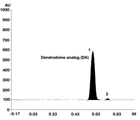
Fig. (2). Peak showing the purity profile of DA as analyzed using HPTLC.
