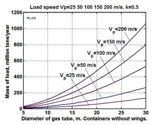
**Fig. (11).** Load delivery *via* the tube diameter and speed payload by wingless containers for k=0.5. Delivery by winged container may be some times more. The load delivery of a conventional two-line railroad is about only 15-30 million tons/year. But a railroad's capital cost is more expensive by many times than the offered high-speed aerial transport system. The big (diameter 1.4 m) oil pipeline has delivery capability of about 100 million tons/year.
