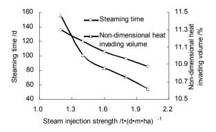
Fig. (5). The influence of steam injection strength on steam breakthrough.
