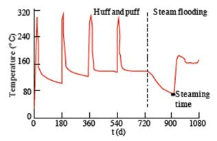
Fig. (1). The temperature profiles of the bottom of producer .
