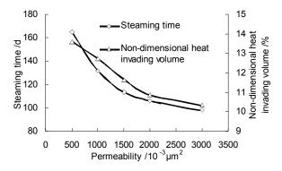
Fig. (3). The influence of permeability on steam breakthrough.
