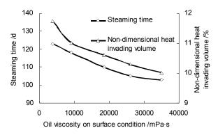
Fig. (4). The influence of oil viscosity on steam breakthrough.
