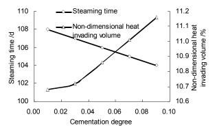
Fig. (6). The influence of cementation degree on steam breakthrough.
