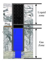
Fig. (1). The schematic of ideal wellbore model during bullheading process.
