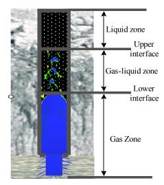
**Fig. (2).** The schematic of three zones partition during bullheading process.
