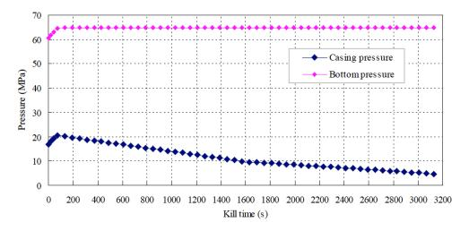
Fig. (4). The calculated results in terms of observed well casing and bottom pressure.
