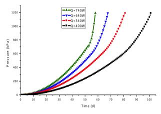
Fig. (7). Laws of lossless storage under different heat leakages.
