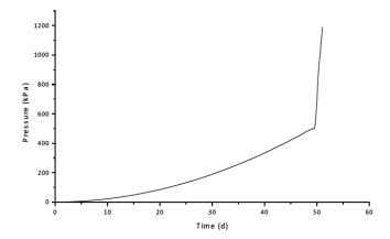
Fig. (4). Pressure changes with time during the storage in the fullness rate of 95%.
