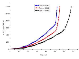
Fig. (8). Laws of lossless storage under different ambient temperatures.
