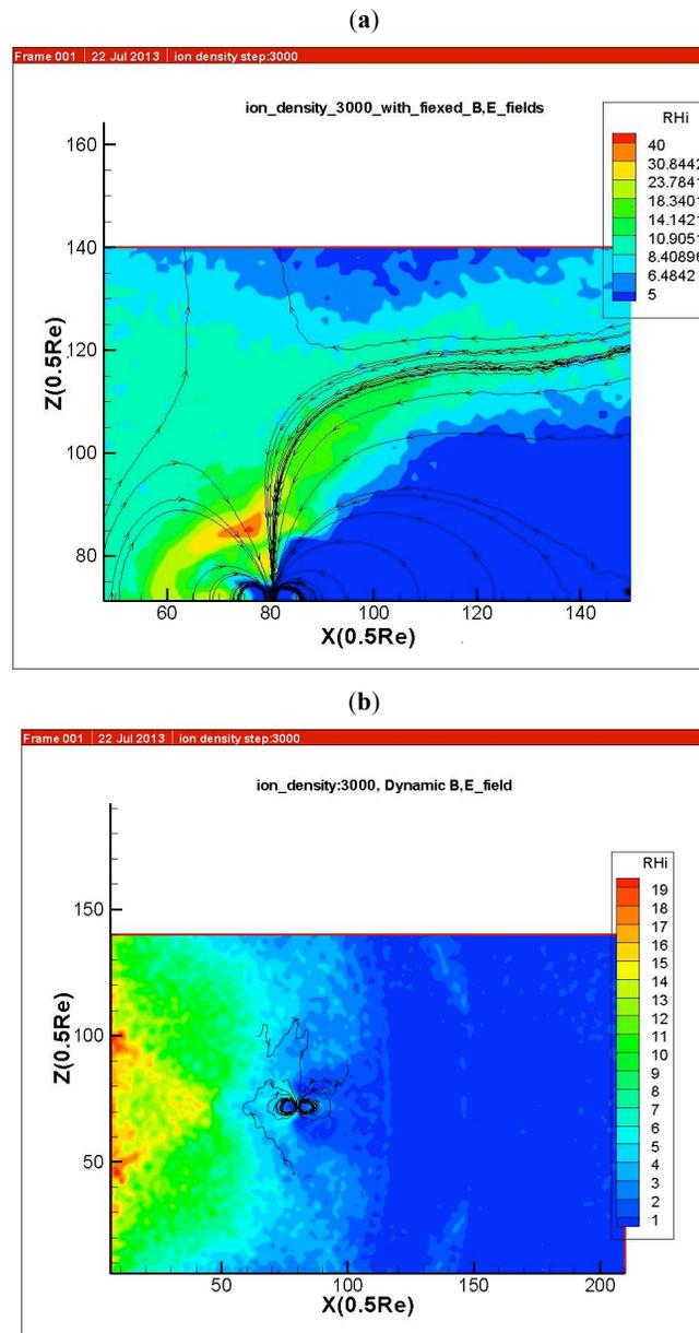
**Fig. (4).** Results of Test particle method with the initial EM fields of 2500 time step and about  $3 \times 10^6$  electron-ion pairs for cases of **a)** static EM fields, **b)** dynamic EM fields.
