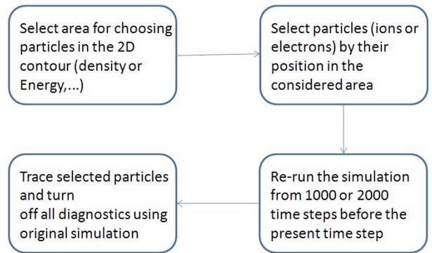
**Fig. (3).** Diagram of particle tracing method in PIC simulation. (EM) fields and dynamic fields were considered. The same number of particles used in the tracing method was used for
