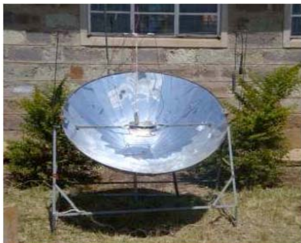
Fig. (4). Processing A. secundiflora sap using a domestic parabolic solar cooker.
