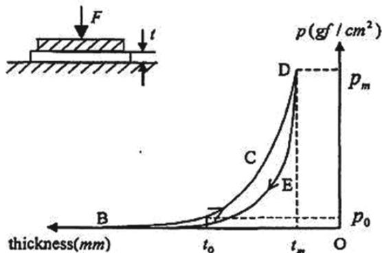
Fig. (2). KES compression measurement: Typical pressure-thickness curve for fabric in lateral compression.
