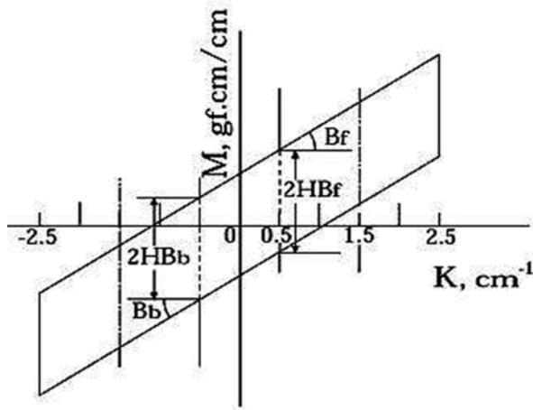
Fig. (1). KES bending measurement: Typical bending moment-curvature curve for fabric in forward and backward direction.
