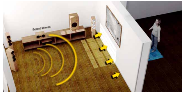
Fig. (4). Occlusion example. The direct path between the sound source and the listener is occluded by the wall. Despite the absence of the direct path, sound can still reach the listener indirectly via diffraction.
