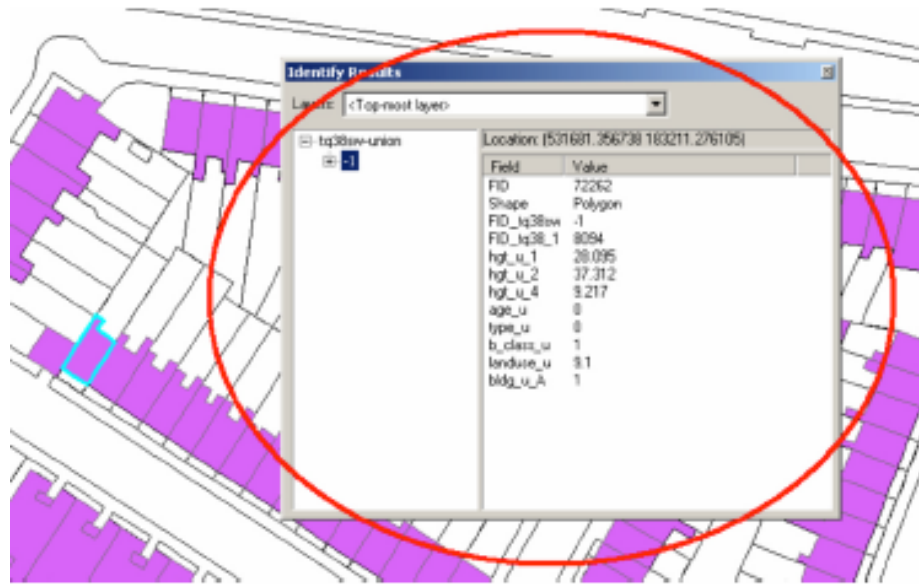
Fig. (2). shp attributes for a single London building, containing key values for reconstruction such as height(s), age and land use.
