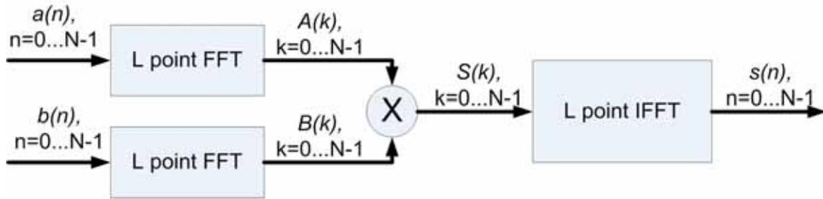
Fig. (2). Block diagram of the cyclic convolution calculation in frequency domain.
