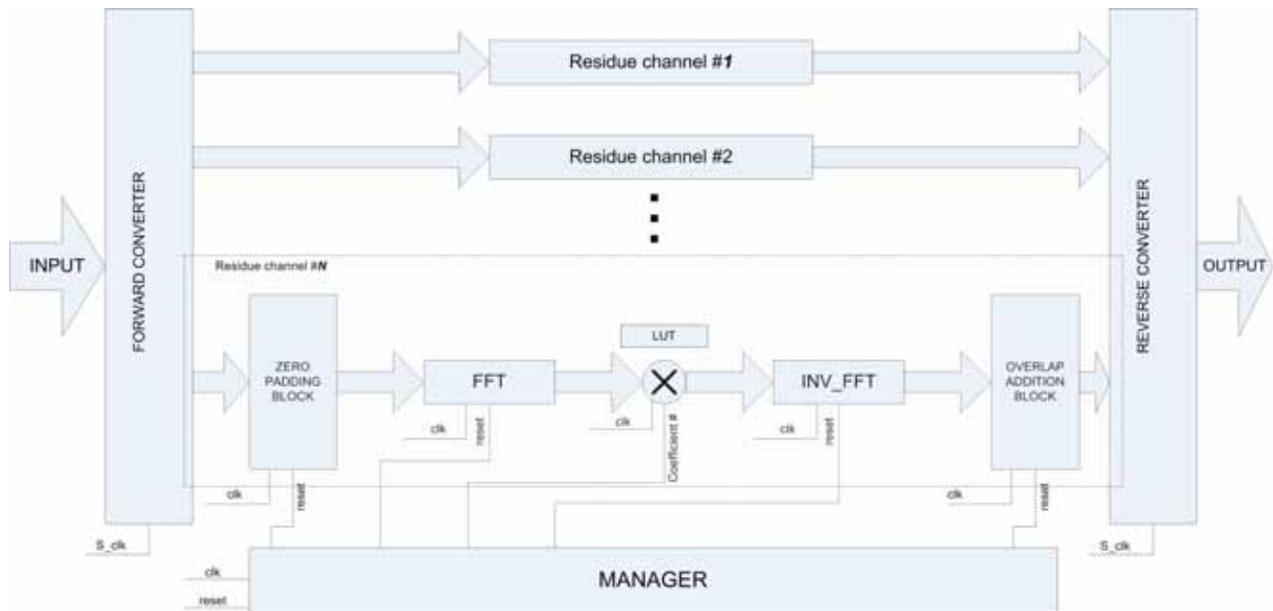
Fig. (3). Block schematic diagram of FIR filter in frequency domain.
