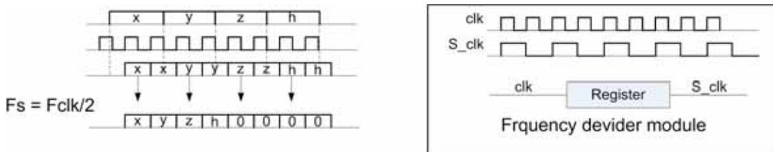
Fig. (4). Zero padding block and frequency divider block.
