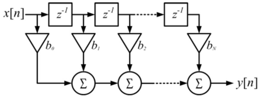
Fig. (1). Canonical form of FIR filter.
