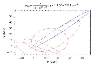
**Fig. (20).** Section in the coordinate {XY} plane of the numerically integrated orbits of an Oort comet with a=66.6 kAU, e=0.92, I=81 deg. Dashed blue line: Newton. Dash-dotted red line: MOND with  $\mu_{3/2}$ ,  $\eta=1.5$  (V=220 km s<sup>-1</sup>). The initial conditions are  $x_0=40$  kAU,  $y_0=30$  kAU,  $z_0=5$  kAU,  $\dot{x_0}=-23$  kAU Myr<sup>-1</sup>,  $\dot{y_0}=-15$  kAU Myr<sup>-1</sup>. The time span of the integration is  $-P_b \le t \le 0$ .
