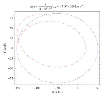
**Fig. (6).** Numerically integrated orbits of an Oort comet with  $a=100\,$  kAU, e=0.5,  $P_{\rm b}=31.6\,$  Myr. Dashed blue line: Newton. Dash-dotted red line: MOND with  $\mu_{3/2}$ ,  $\eta=1.5\,$  ( $V=220\,$  km s  $^{-1}$ ). The initial conditions are  $x_0=-a(1+e), y_0=z_0=0, \dot{x}_0=0, \dot{y}_0=-na\sqrt{\frac{1-e}{1+e}}, \dot{z}_0=0$ . The time span of the integration is  $-P_{\rm b} \le t \le 0$ .
