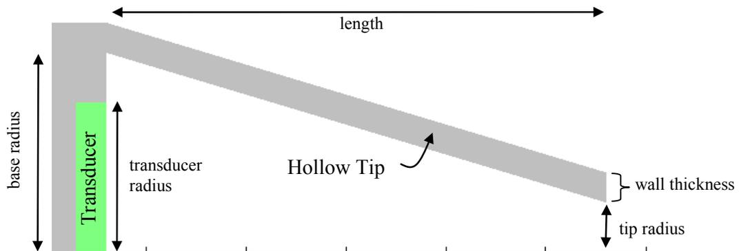
Fig. (8). A linear tip and its parameterized dimensions.
