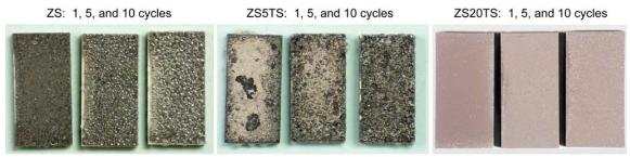
Fig. (2). Macrophotos of coupons after oxidation at 1627°C in stagnant air.
