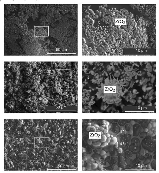
**Fig. (3).** Secondary electron images showing surface morphology of the ZS (top), ZSTS5 (middle), and ZSTS20 (bottom) after oxidation at 1627°C for 100 min in stagnant air. Details of area in white box on left are shown in higher magnification on the right. ZrO<sub>2</sub> and glass (g) phases are labeled in the right hand micrographs. Note that only the ZSTS20 shows evidence of immiscible glass formation: g1 is silica rich while g2 contains Al and Mg impurities.
