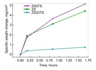
Fig. (1). Weight change results obtained at 1627°C in stagnant air for ZrB<sub>2</sub>-20 v% SiC baseline material compared to compositions containing 5 and 20 v% TaSi<sub>2</sub>. ZS and ZS20TS from ref. [9].
