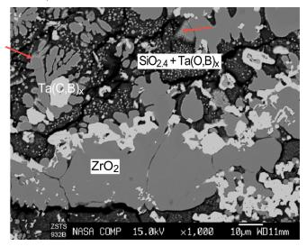
**Fig. (10).** Backscattered electron image of the middle of the oxide scale formed on ZSTS20 after oxidation at 1927°C for five 10-minute cycles in stagnant air. Same area as Fig. (9). The red arrows highlight the bright contrast surface layer found on zirconia suggesting Ta-enrichment.
