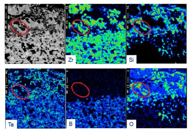
Fig. (8). Backscattered electron image and corresponding WDS dot maps for the substrate/oxide interface of ZSTS20 after oxidation at 1927°C for five 10-minute cycles in stagnant air. The red oval focuses on an area containing ZrO2, SiO2, and micron-sized, Ta-rich oxyboride phases.
