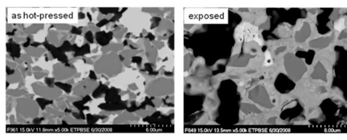
**Fig. (6).** Backscattered electron image of ZSTS20 substrate before and after oxidation for 50 min at 1927°C in stagnant air. Four phases are present in the hot-pressed material (from brightest to darkest contrast):  $TaSi_2$ ,  $(Zr,Ta)B_{1.5}$ ,  $ZrB_2$ , and SiC. The exposed sample contains (from brightest to darkest contrast)  $(Zr,Ta)C_x$ ,  $(Zr,Ta)B_x$ ,  $ZrB_2$ , SiC and porosity.
