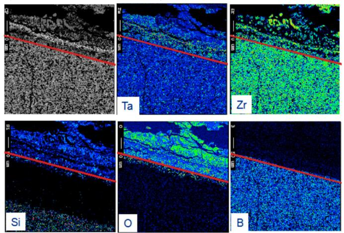
Fig. (7). Backscattered electron image and corresponding WDS dot maps for the substrate/oxide interface of ZSTS20 after oxidation at  $1927^{\circ}$ C for five 10-minute cycles in stagnant air. The red line corresponds to the approximate location of the  $ZrO_2/ZrB_2$  interface as discussed in the text.
