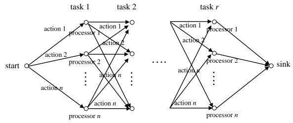
Fig. (1). The graph representation of the TAP as a reinforcement learning network.
