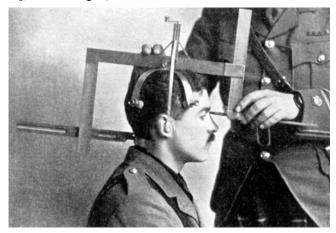
**Fig. (6).** An anthropometric device (side view) by Major A.J.N. Tremearne designed "for measuring the living head" for "the use of anthropologists", invented in 1913 with later additions (modified from Tremearne 1914 [91]).
