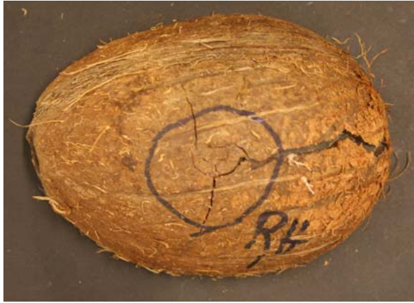
Fig. (6). Coconut struck by round hammer (Fig. 2) showing impression fracture and fracture lines.
