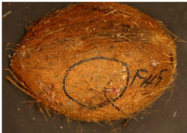
Fig. (7). Coconut struck with a square hammer (Fig. 3) showing a V-shaped impression fracture matching the square hammer in size and shape. Furthermore a fracture line is seen.
