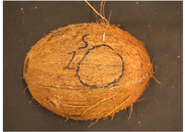
Fig. (8). Coconut struck with a crescent wrench (Fig. 4) showing an impression fracture matching the pin of the wrench in shape and size. There are no fracture lines.
