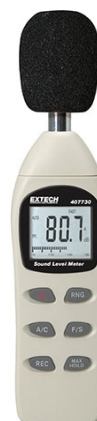
Fig. (7). This sound level meter from Extech (Model 407730) measures sound intensity from 40 to 130dB SPL with an accuracy of 2dB. More information on this unit is available at http://www.extech.com/resources/407730_DS-en.pdf . Image Credit: http://www.extech.com/images/407730.png .
