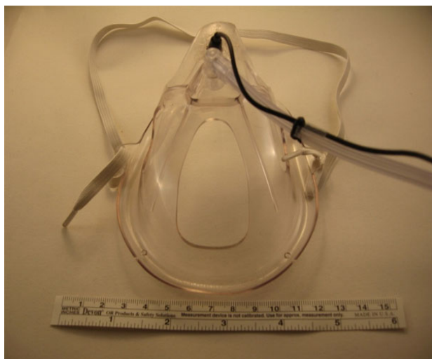
Fig. (4). A miniature electret microphone embedded into an oxygen mask can be used to record breath sounds.
