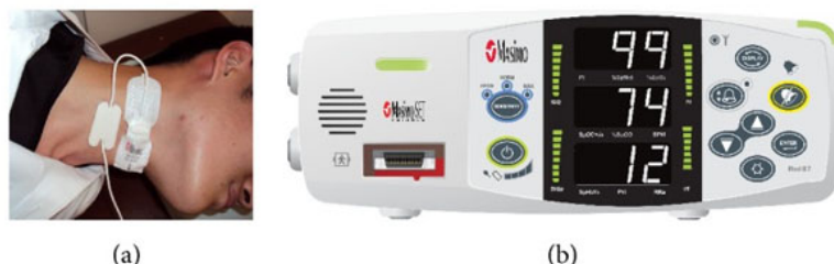
Fig. (3). Acoustic respiratory rate monitoring device from Masimo. (a) Acoustic monitoring sensor placed on the neck via an adhesive coating. (b) The display (Masimo Rad-87) showing arterial oxygen tension, heart rate and respiratory rate respectively. Image used under a Creative Commons Attribution License 4.0 from Suzuki T, Tsuda S, Nakae H, et al. Usefulness of Acoustic Monitoring of Respiratory Rate in Patients Undergoing Endoscopic Submucosal Dissection. Gastroenterol Res Pract. 2015;2016:2964581.PMID: 26858748.
