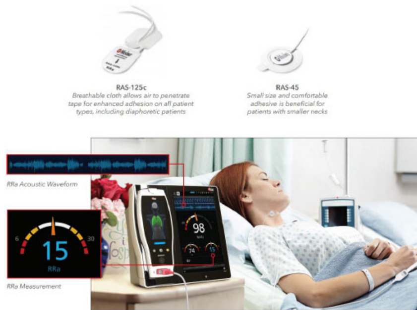
Fig. (8). The Masimo system for acoustic respiratory rate monitoring is a well-established technique for respiratory monitoring. Two forms of available acoustic sensors are available, and both are designed for placement on the neck, near the trachea. The system also includes a pulse oximetry feature, and numerically displays the arterial oxygen saturation, the heart rate and the respiratory rate (known as RRa). Also displayed is the time-domain acoustic waveform, a feature that can be helpful when troubleshooting. While multiple studies have confirmed the value of this method of acoustical respiratory monitoring in a number of settings, the technology as currently available has some important limitations. First, neither the raw nor the processed acoustic signal is available to the clinician to listen to, although the time-domain signal is displayed. The fact that the system does not provide an analog signal output for such purposes also limits the kind of supplementary analysis that might otherwise be performed, such as digitally recording the obtained signals, subjecting the signal to analog or digital filtering, or carrying out real-time color spectrographic analysis of the obtained breath sounds. Also, because of the proprietary nature of the Masimo acoustic monitoring system, little is publicly known about the flat acoustic sensor used. The likelihood, however, is that their sensor is based on piezoelectric film technology, as this technology has proven to be very useful in a variety of clinical applications. Image Credit: http://www.masimo.com/siteassets/us/documents/pdf/plm-10023b_product_information_rra_us.pdf
