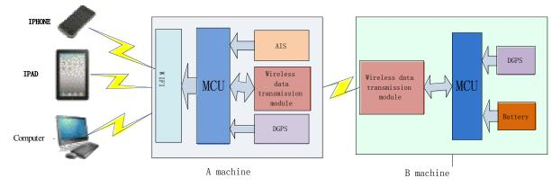
Fig. (1). Hardware diagram of berthing system of large vessels.
