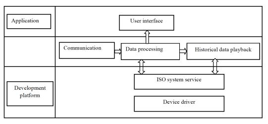
Fig. (2). The structure of software system.
