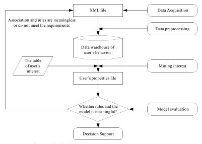
Fig. (4). Model of data mining system of users' behavior.
