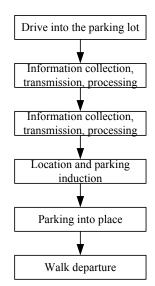
Fig. (4). Parking guidance system flow.
