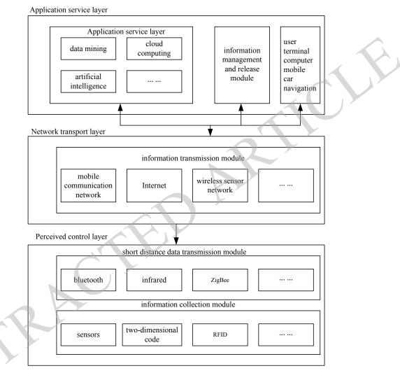
Fig. (1). The framework of Basement Parking Intelligent Monitoring System based on the internet of things.
