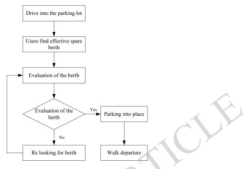
Fig. (3). Parking flowchart artificial guide.
