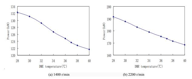
Fig. (3). Effect of DME temperature on power of DME engine (injection advance angle 8°CA BTDC, P8500 Pump, 12 mm piston,  $6 \times 0.43$  mm nozzle).
