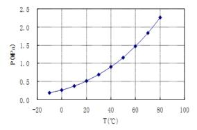
Fig. (5). Effect of temperature on vapor pressure of DM.
