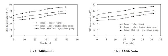
Fig. (2). Variation of DME temperature with time (injection advance angle  $8^{\circ}$ CA BTDC, P8500 Pump, 12 mm Piston,  $6 \times 0.43$  mm Nozzle).
