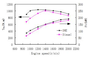
**Fig. (1).** Comparison of torque and power of DME engine and diesel engine at full load.
