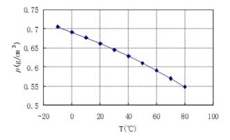
Fig. (4). Effect of temperature on Density of DME.
