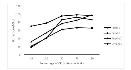
Fig. (3). CPU utilization rate with the ratio of CPU-intensive tasks.
