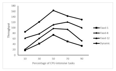
Fig. (5). System throughput with the ratio of CPU-intensive tasks.
