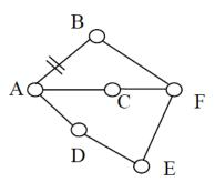
Fig. (1). Schematic diagram on concept of post-earthquake road section connectivity.
