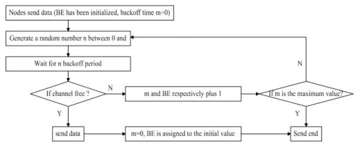
Fig. (6). The CSMA/CA algorithm flow.
