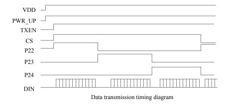
Fig. (3). The data transmission time sequence.
