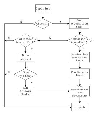
Fig. (7). Sample collection and logic diagram.
