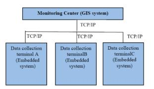
Fig. (1). Total system framework map. TCP means transmission control protocol, ip means internet protocol.
