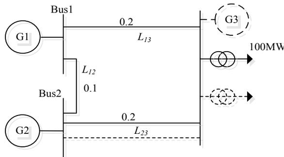
Fig. (2). Three-bus power system.
