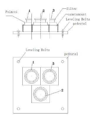
Fig. (3). Schematic diagram of detection device.
