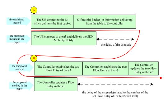
Fig. (11). The difference comparison of the handover delay. The difference comparison (2).
