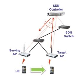
Fig. (1). The handover delay of the SDN network.
