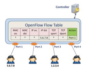
Fig. (2). The framework of the SDN.
