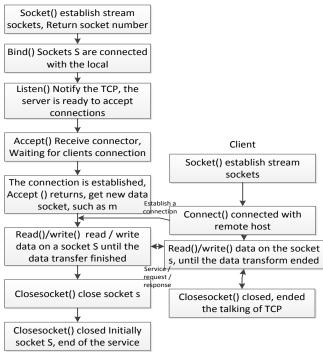
Fig. (3). Using the TCP Protocol Client / Server Mechanism.
