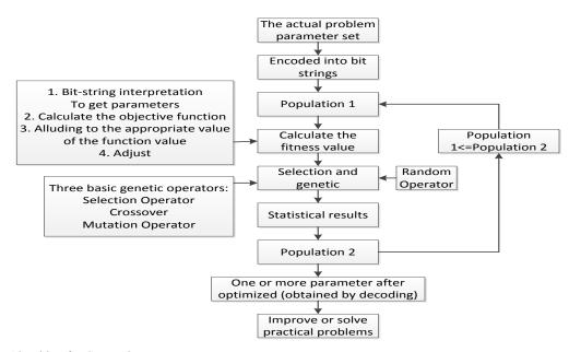
Fig. (2). Genetic Algorithm for Computing Processes.
