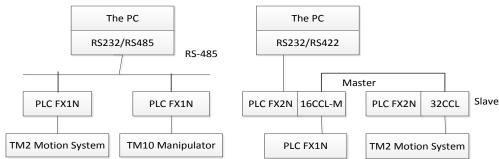
Fig. (1). Based on RS-485 and Based on CC-Link.
