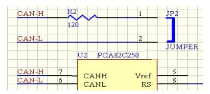
Fig. (6). Resistive circuit loaded in terminal of CAN bus.
