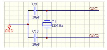
Fig. (5). Crystal circuit of Mcp2515.
