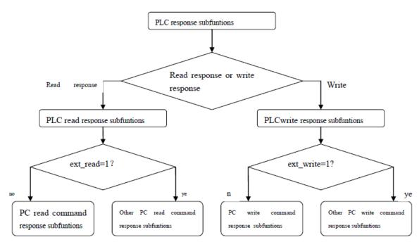
Fig. (9). Flow chart of PLC response subfunctions.
