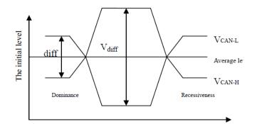
Fig. (1). Level of value logic of CAN bus.
