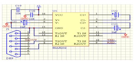
Fig. (3) Serial interface circuit.
