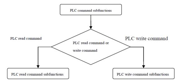
Fig. (8). Flow chart of PLC command subfunctions.
