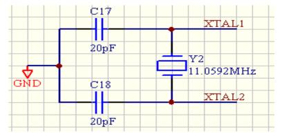
Fig. (4). Crystal circuit of Atmega8.
