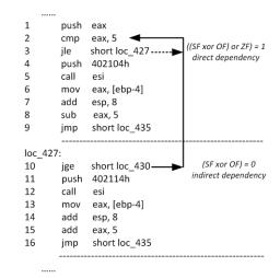
Fig. (3). An example of invertible analysis of some part of instructions from a binary file.
