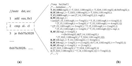
Fig. (1). A simplified example of a three line assembly program is shown on the left (a). The right (b) illustrates the statement of the second instruction *cmp*.
