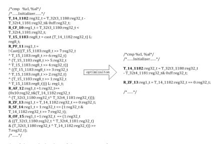
Fig. (4). A simplified example of the optimization of the statement of *cmp*.
