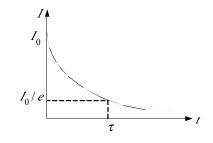
Fig. (1). Fluorescence decay curve.
