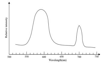
**Fig. (4).** The spectrum of exciting light of LED *via* sensor probe  $(Cr^{3+}: Al_2O_3)$ .
