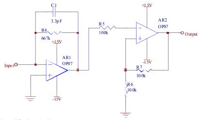
Fig. (6). Fluorescence signal amplification circuit.
