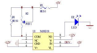
Fig. (5). Schematic of the LED drive circuit.
