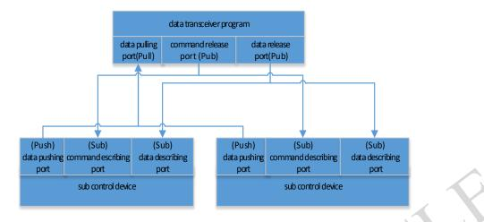
Fig. (3). ZeroMQ communication mode designing.
