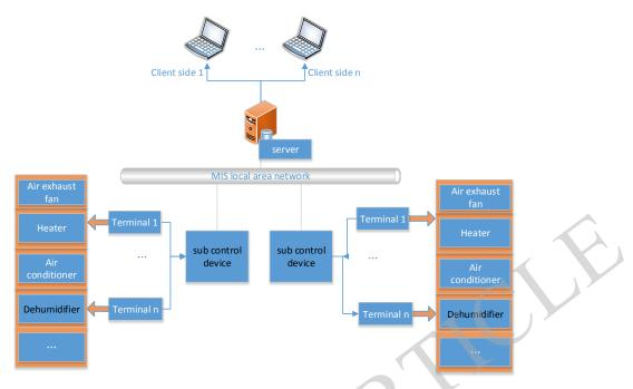
Fig. (1). The overall diagram of temperature and humidity monitoring system.
