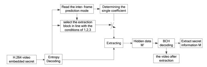
Fig. (4). The Extracting Operation Process of Single Coefficient BCH Robustness Method.
