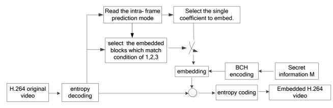
Fig. (3). The Embedding Operation Process of Single Coefficient BCH Robustness Method.
