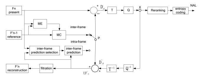
Fig. (1). H.264/AVC Coding Process Structure.
