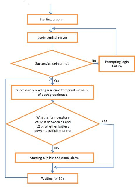
Fig. (3). Temperature warning algorithm flow chart.
