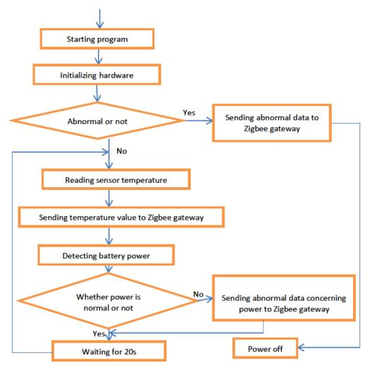
Fig. (2). Temperature detecting algorithm flow chart.
