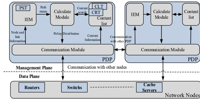
Fig. (1). PDP block diagram.
