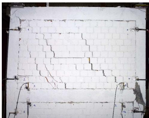
Fig. (1.1). Crack pattern of a sheared planar wall in reinforced concrete frame (photo: second author).
