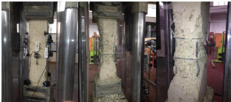
**Fig. (11).** Columns of the first series: steel rebars type B.
