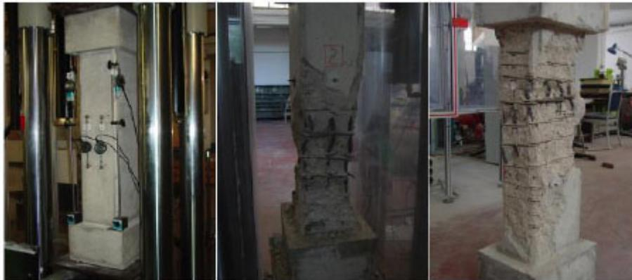
**Fig. (10).** Columns of the first series: steel rebars type A.
