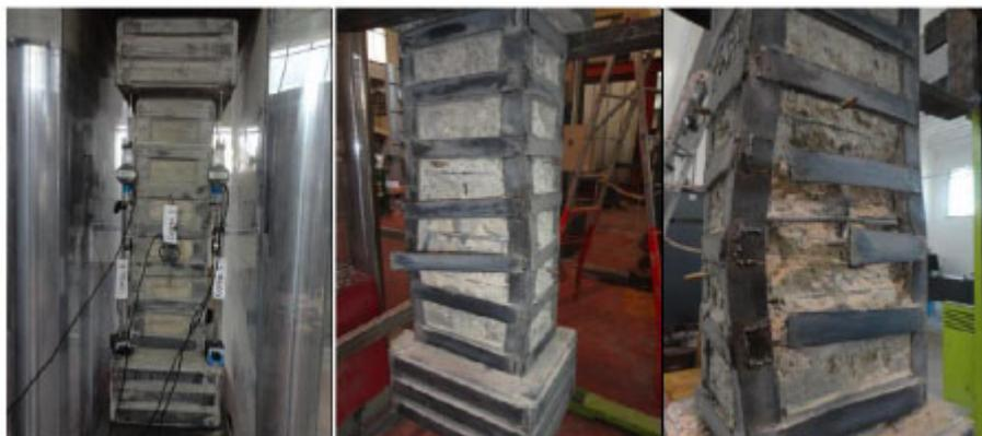
**Fig. (12).** Strengthened columns: steel rebars type B.
