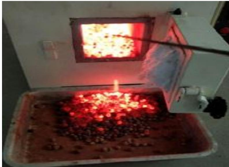
**Fig. (2).** Burning aggregates in muffle furnace.
