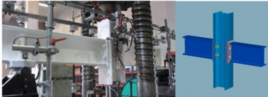
Fig. (4). Layout of the EPB connection.
