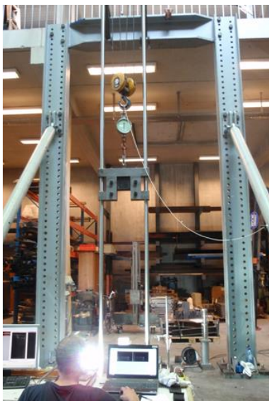
Fig. (8). Testing setup for the impact tests.
