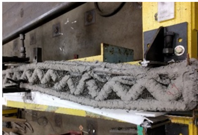
Fig. 11. Mode of failure for beams 2DR-S-6B and 3DR-S-6B: Shear failure at nodal points.
