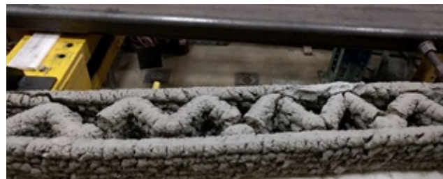
Fig. (13). Mode of failure for beam 4DR-S-0: Shear failure due to nodal detachment near beam supports.
