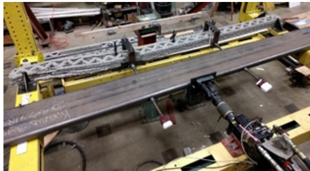
Fig. (5). Third-point bending test setup, looking toward negative y.
